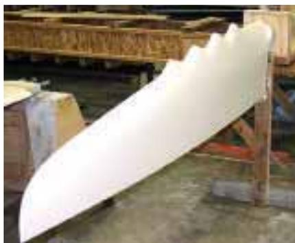
**Above:** Bieker's rudder tubercles act to provide better control for a given foil size. **Left:** hard chines allied to relatively soft aft sections ensure that for such a powerful design Paul Bieker's latest offshore creation still slides along easily in light air
