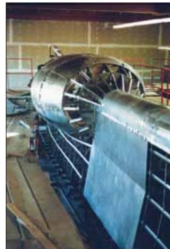
**Left**—Other than high-performance sailboats, Betts has done a few builds such as this 78' (24m) SWATH, which rides on submerged torpedo-like hulls for improved sea-keeping. Their construction in aluminum is shown at **right**.
