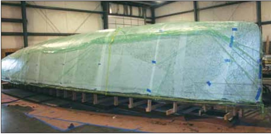
The 39' (12m) *Bien Roulée*, an Alan Andrews-designed racer, seen **above** on the male plug, and at **right** turned right side up with the sail drive foundation installed, was built in 2007 of carbon and Corecell. Betts works only with epoxy resins, citing their environmental and structural advantages.
