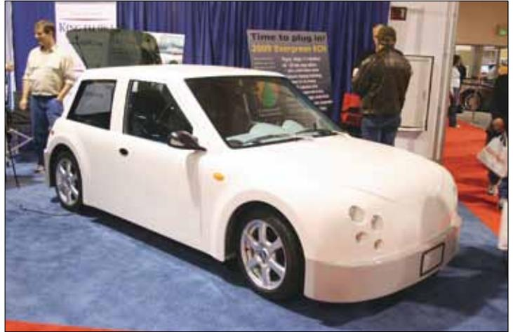
**Left**—Betts’s son Kellen designed this electric car for a client on Bainbridge Island, Washington, who wanted to series-produce it under the Neighborhood Electric Vehicle Law, which doesn’t require crash testing. The NEV speed limit is 35 mph (56 kmh), though it can go faster. **Right**—It was exhibited at the 2009 Seattle Auto Show; the body and chassis are carbon composite.
