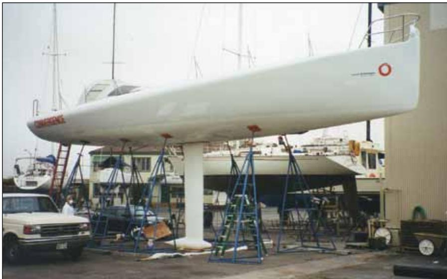
*Convergence, an Open 50 that sailed in the 2002 Around Alone race under the name Everest Horizontal, is one of two composite boats Betts has built with balsa core—in this case, to provide buoyancy.*
