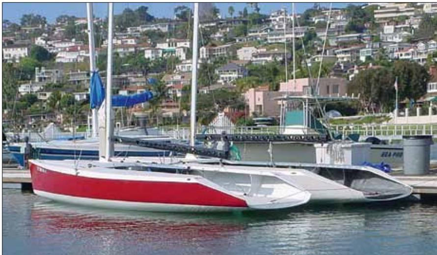
One of Betts's few forays into series production was the Sierra 26 (7.9m) one-design, built of pre-preg carbon and honeycomb composite, post-cured over an aluminum tool. Just two were built.
